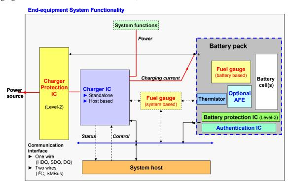
The report classifies battery charger ICs into a five-level hierarchy by integration, topology, algorithm execution, input power sources, and application attributes. Fuel gauge ICs are classified by algorithm execution (intelligence), integration, battery chemistry, cell configuration, and protection and monitoring features.
